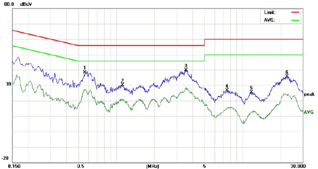
Line Conducted Emission Test Line 1-L
