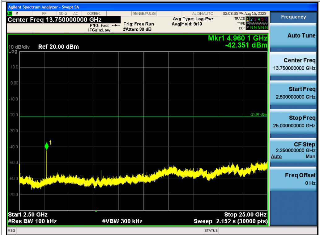
Test_Graph_EDR_ANT1_2480_2Mbps_Higher Band Emissions
