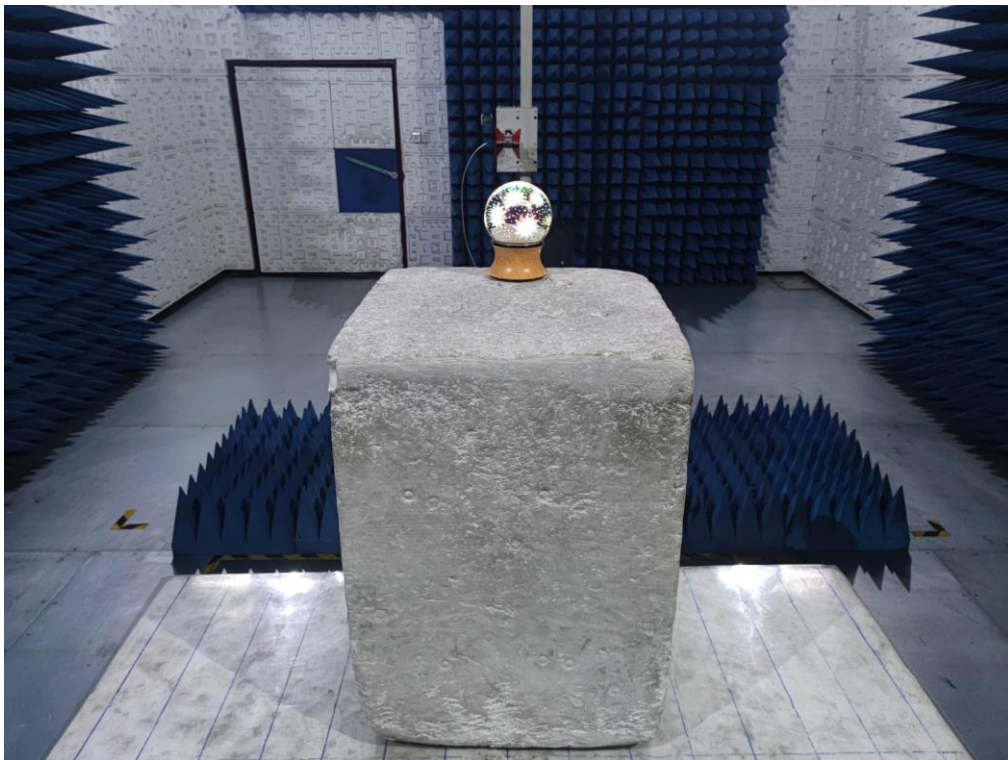
RADIATED EMISSION TEST SETUP ABOVE 1GHz
