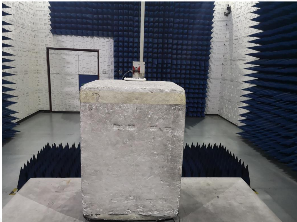
FCC RADIATED EMISSION TEST SETUP ABOVE 1GHZ
