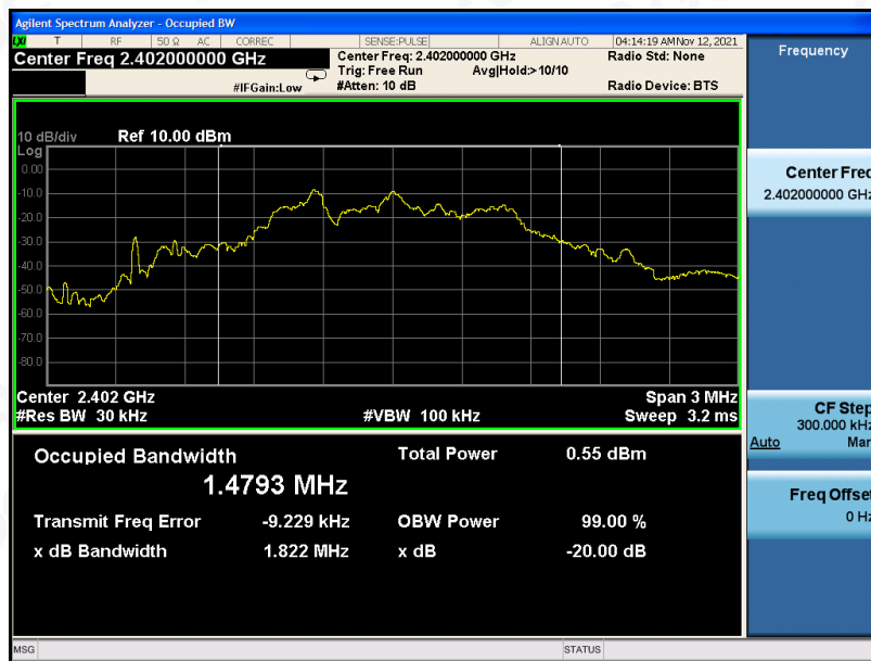
TEST PLOT OF BANDWIDTH FOR LOW CHANNEL
