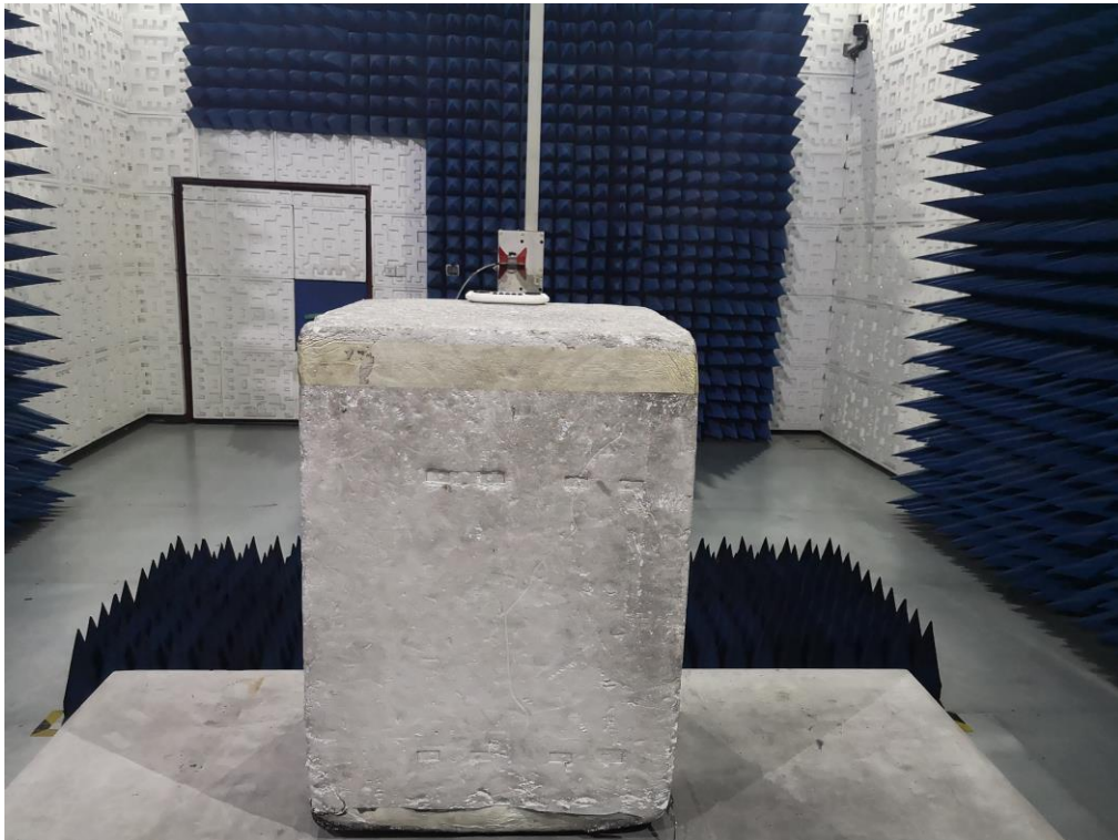
FCC RADIATED EMISSION TEST SETUP ABOVE 1GHZ
