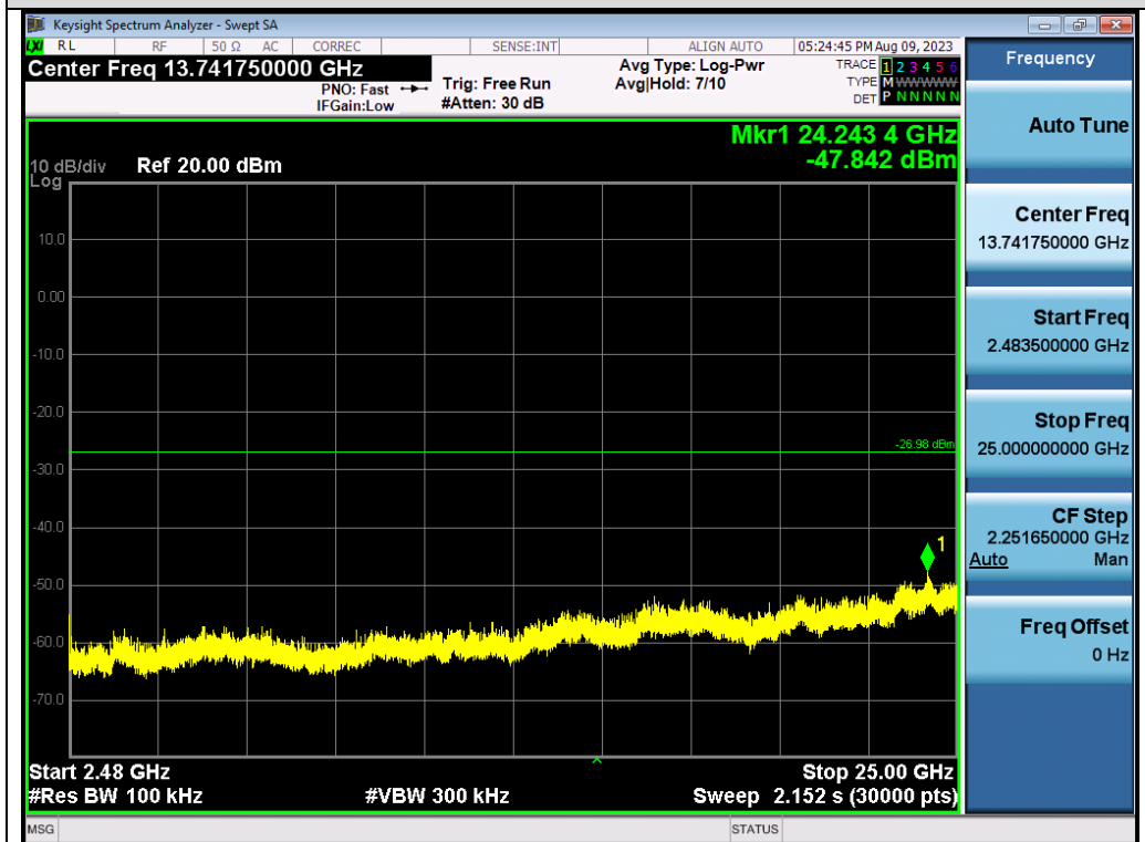
Test_Graph_LE1M_ANT1_2440_1Mbps_Higher Band Emissions
