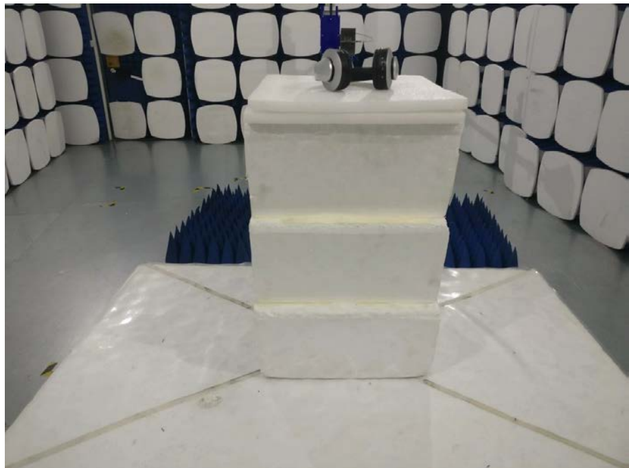
Radiated emission – above 1GHz
