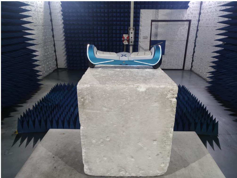
RADIATED EMISSION TEST SETUP ABOVE 1GHz
