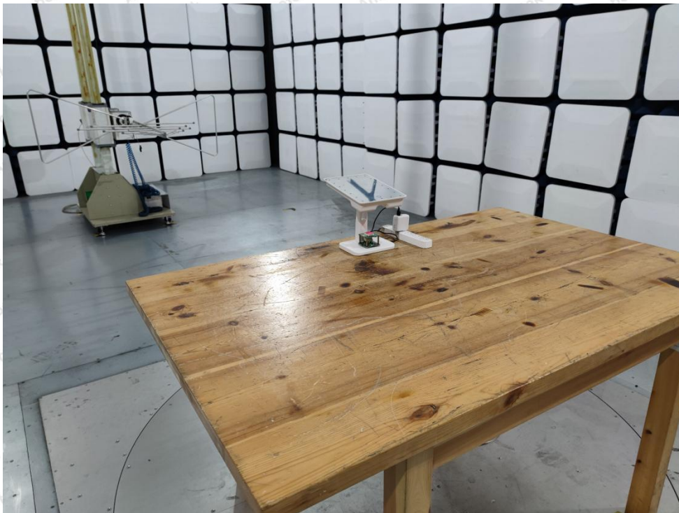
Photo of Radiation Emission Test
