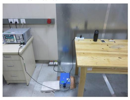
FCC RADIATED EMISSION TEST SETUP
