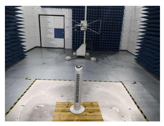
FCC RADIATED EMISSION TEST SETUP ABOVE 1GHZ
