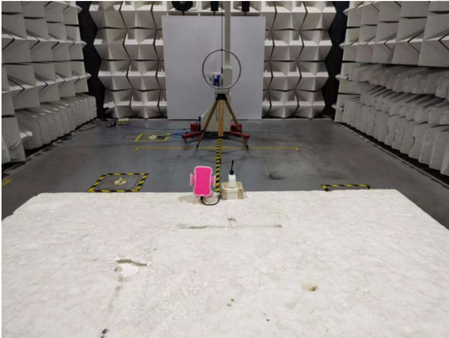
Radiated Spurious Emissions Test Setup-1 (9kHz~30MHz)
