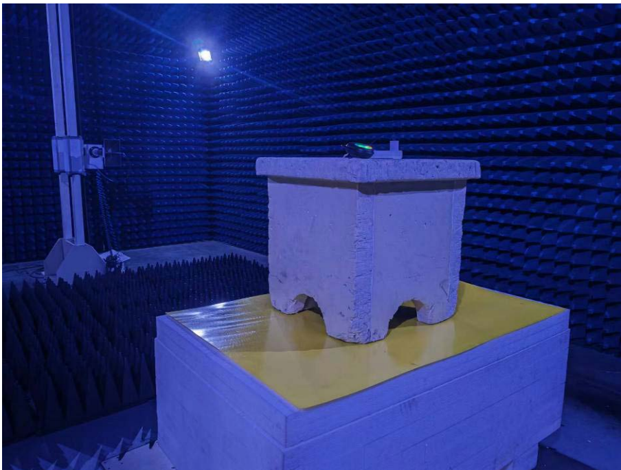
Photo of Radiated Emission Measurement Above 1GHz
