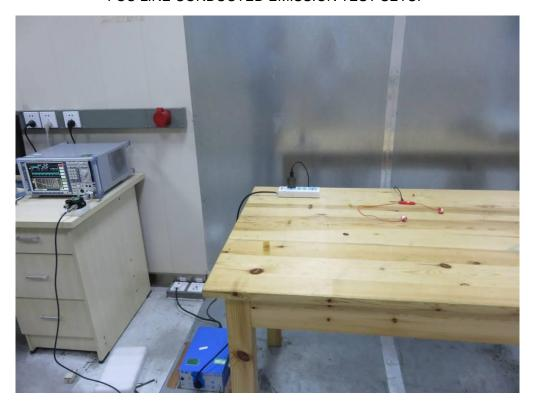
FCC RADIATED EMISSION TEST SETUP
