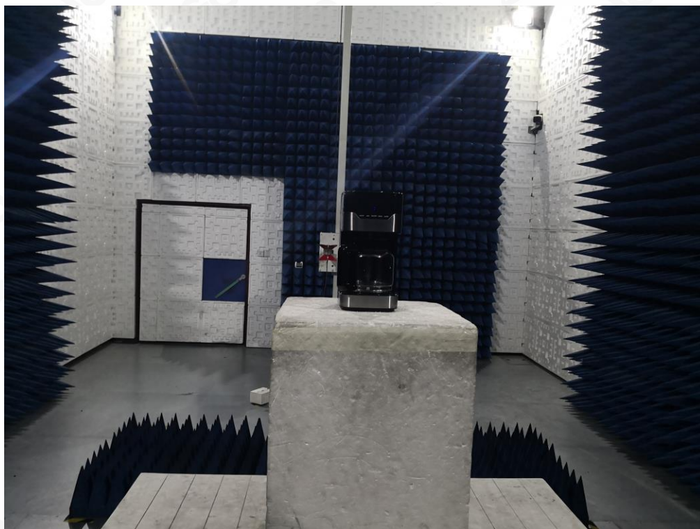
FCC RADIATED EMISSION TEST SETUP ABOVE 1GHZ
