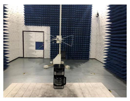
FCC RADIATED EMISSION TEST SETUP ABOVE 1GHZ
