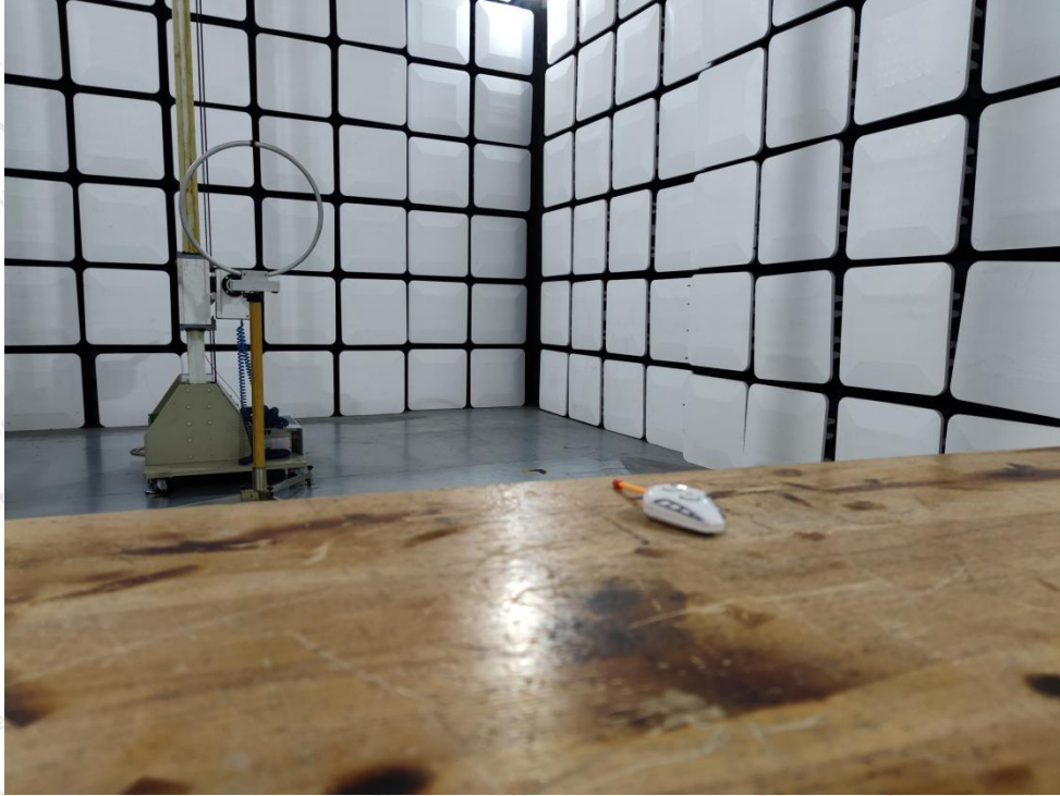
Photo of Radiation Emission Test
