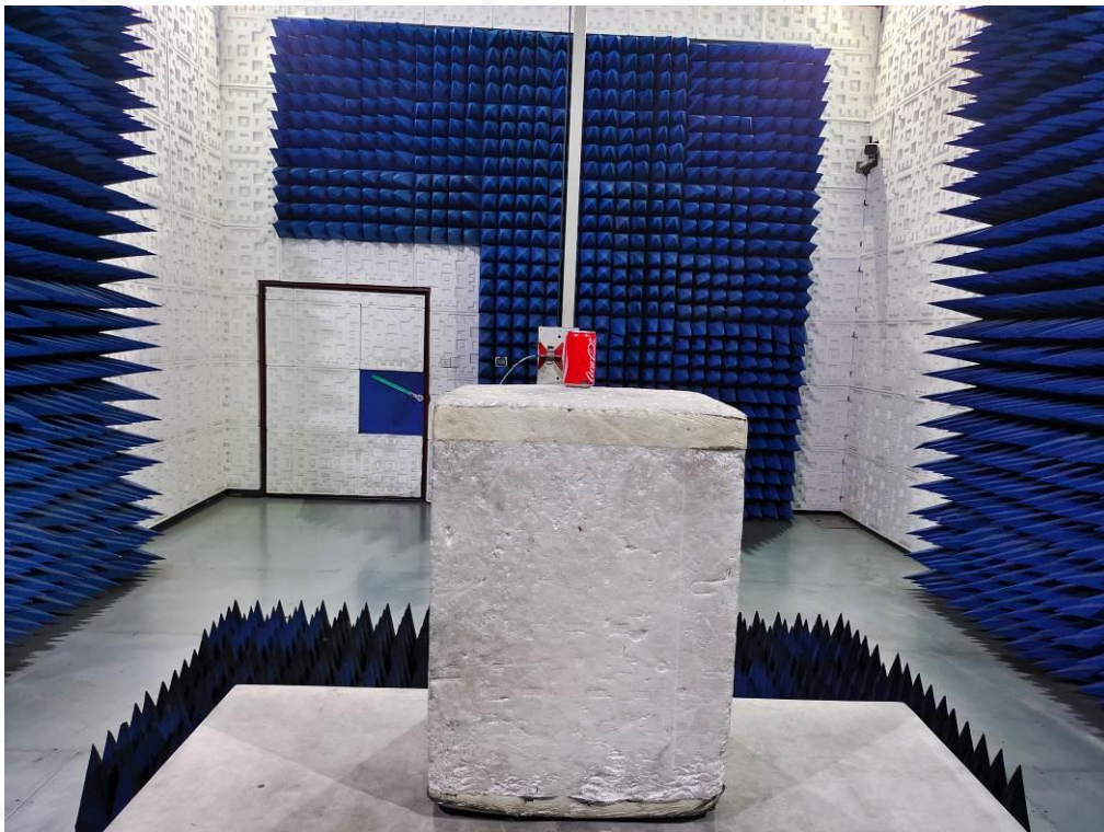
RADIATED EMISSION TEST SETUP ABOVE 1GHZ
