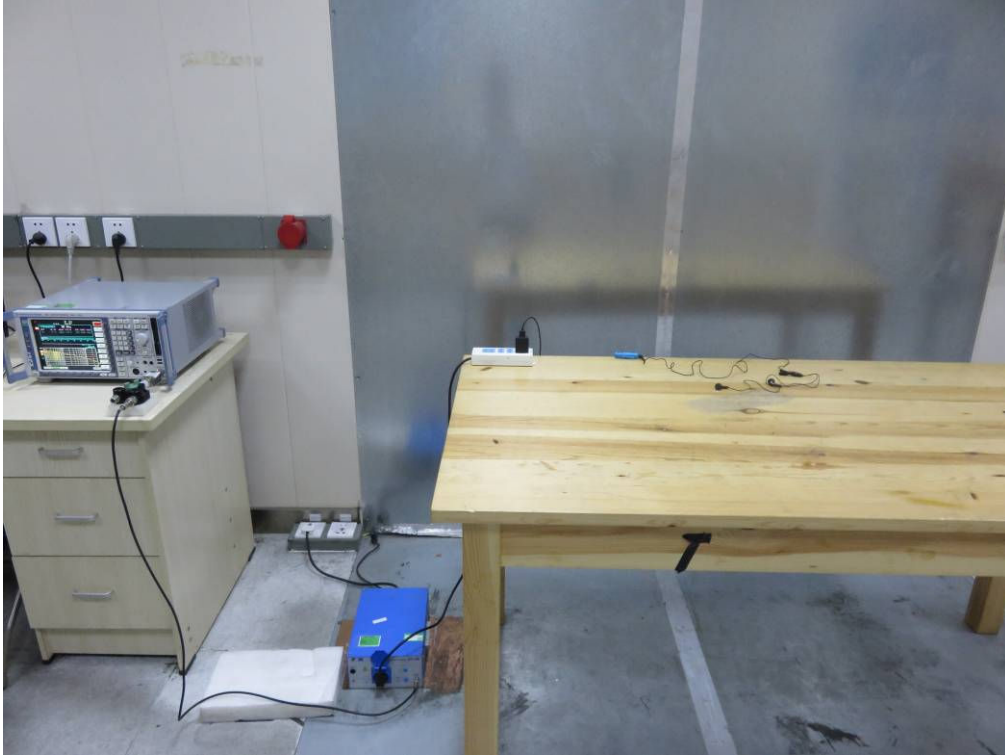
FCC RADIATED EMISSION TEST SETUP
