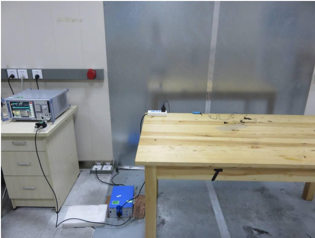
FCC RADIATED EMISSION TEST SETUP
