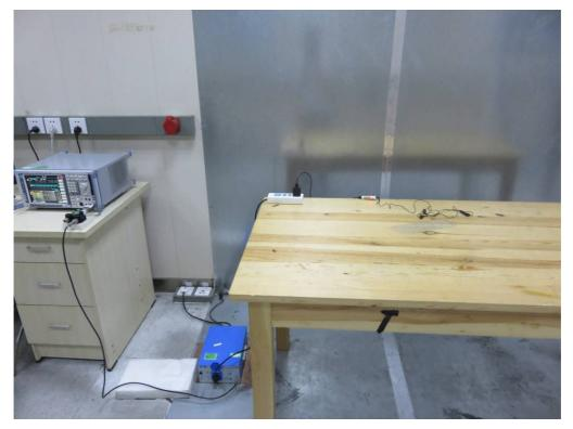
FCC RADIATED EMISSION TEST SETUP
