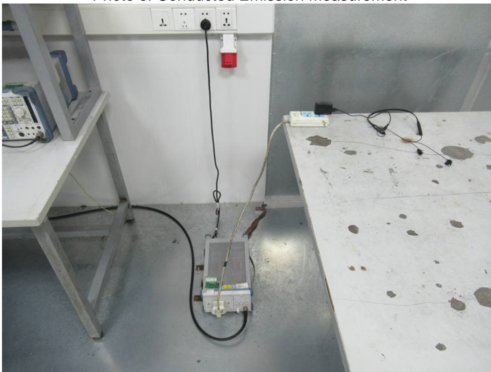
FCC ID: 2AANZBT65 Photo of Conducted Emission Measurement
