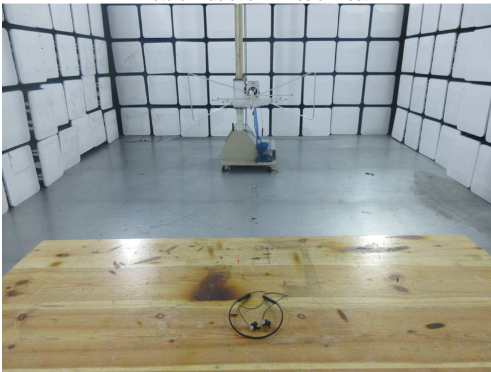
Photo of Radiation Emission Test
