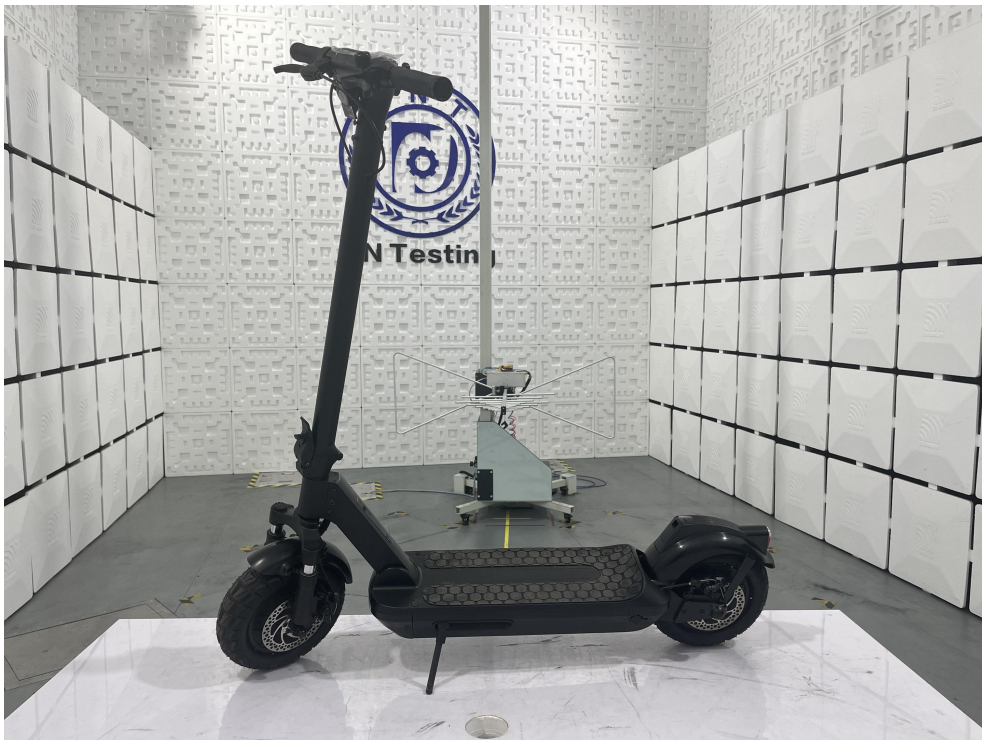
Radiated Emission Test View((Below 1G)
