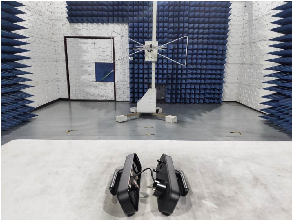
FCC RADIATED EMISSION TEST SETUP ABOVE 1GHZ
