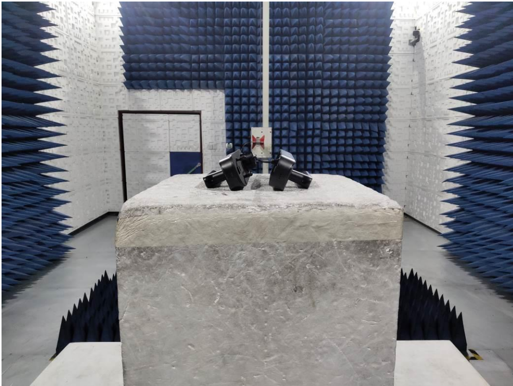
FCC RADIATED EMISSION TEST SETUP ABOVE 1GHZ
