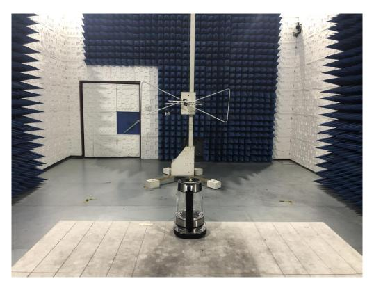
FCC RADIATED EMISSION TEST SETUP ABOVE 1GHZ
