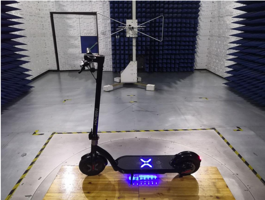
RADIATED EMISSION TEST SETUP ABOVE 1GHZ
