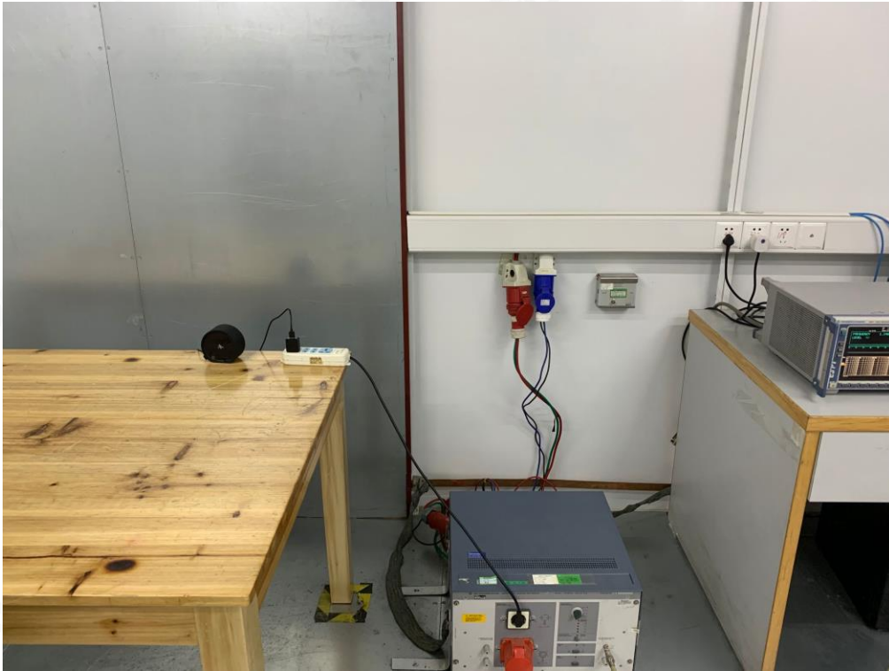
FCC RADIATED EMISSION TEST SETUP BELOW 1GHZ
