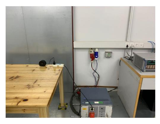
FCC RADIATED EMISSION TEST SETUP BELOW 1GHZ
