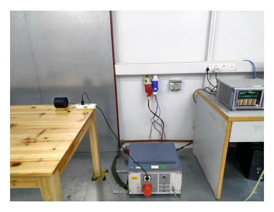
FCC RADIATED EMISSION TEST SETUP BELOW 1GHZ
