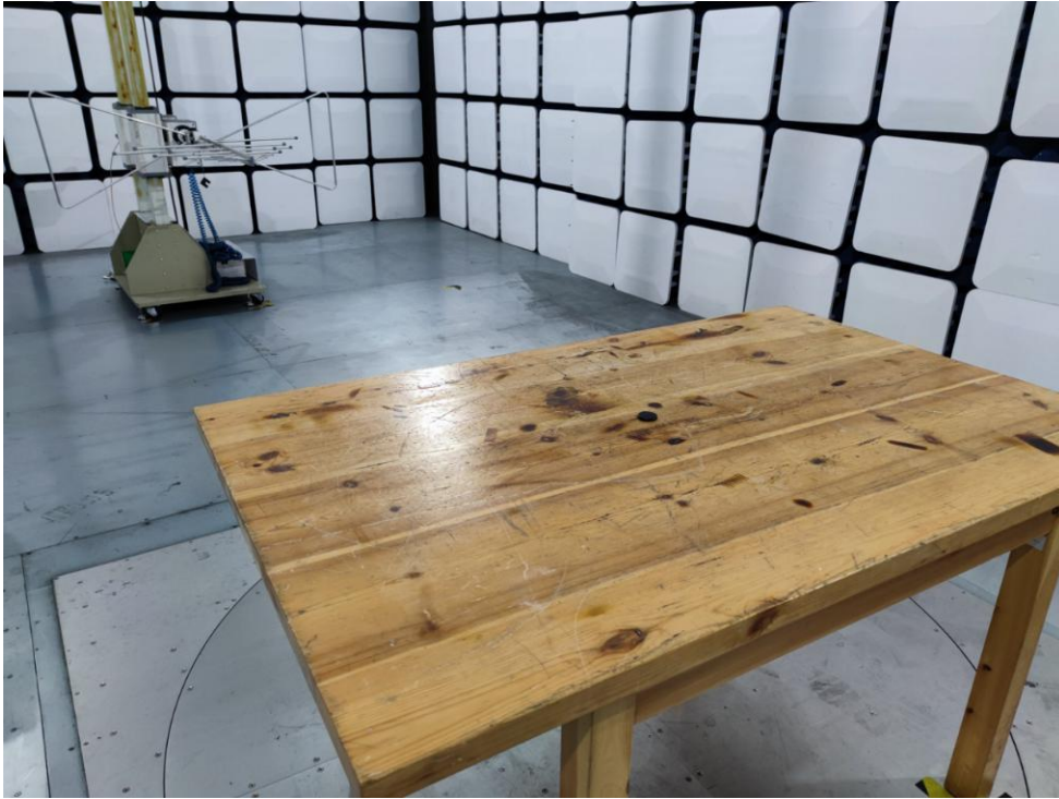
Photo of Radiation Emission Test
