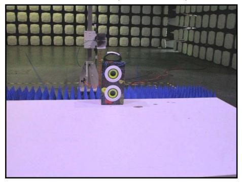
Above 1 GHz: (full anechoic chamber)
