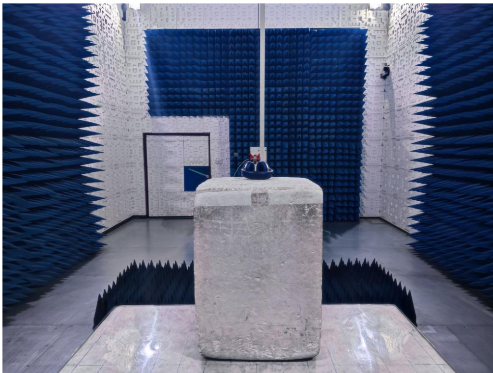
RADIATED EMISSION TEST SETUP ABOVE 1GHZ
