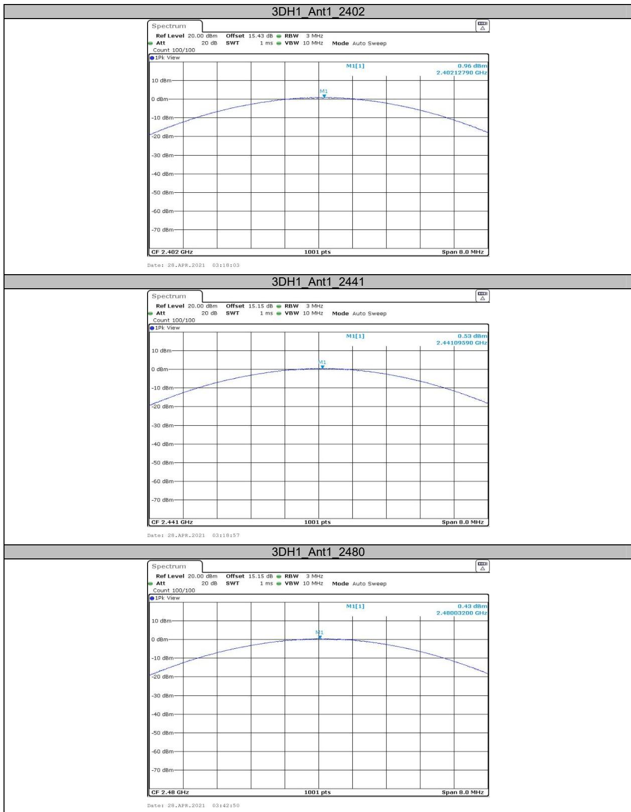
**AppendixC: Carrier Frequency Separation****Test Result**
