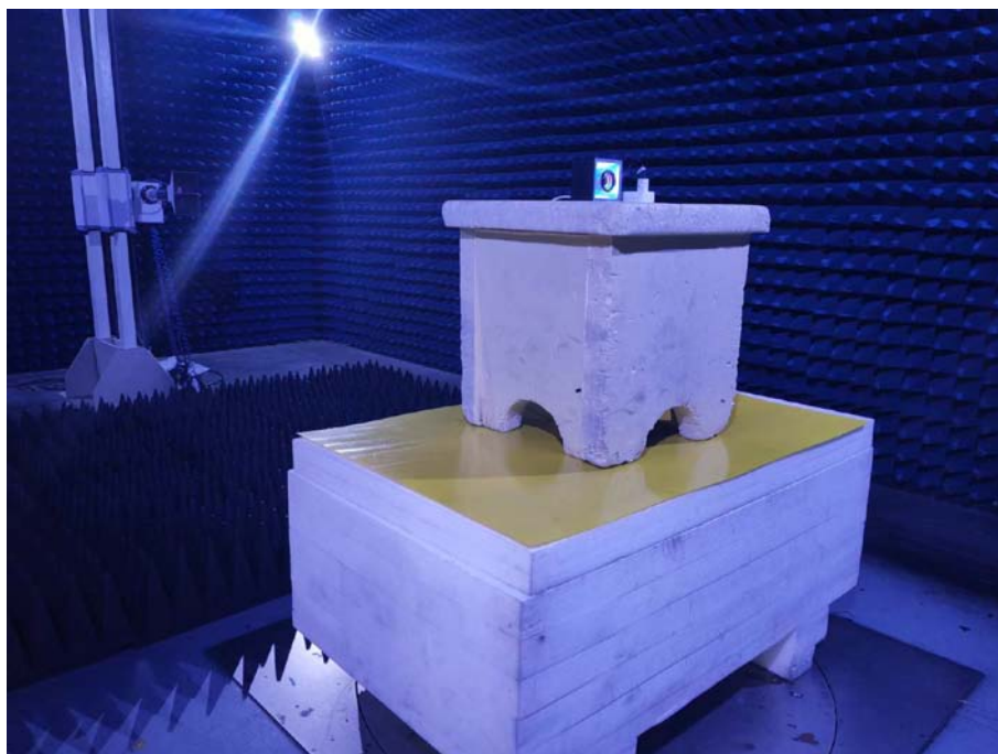
Photo of Radiated Emission Measurement Above 1GHz
