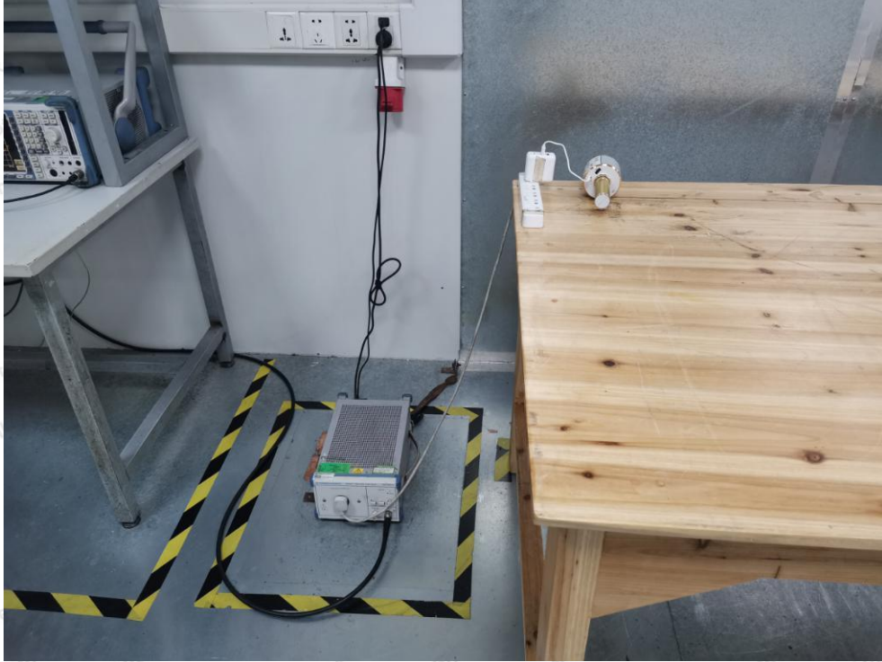
Photo of Conducted Emission Measurement
