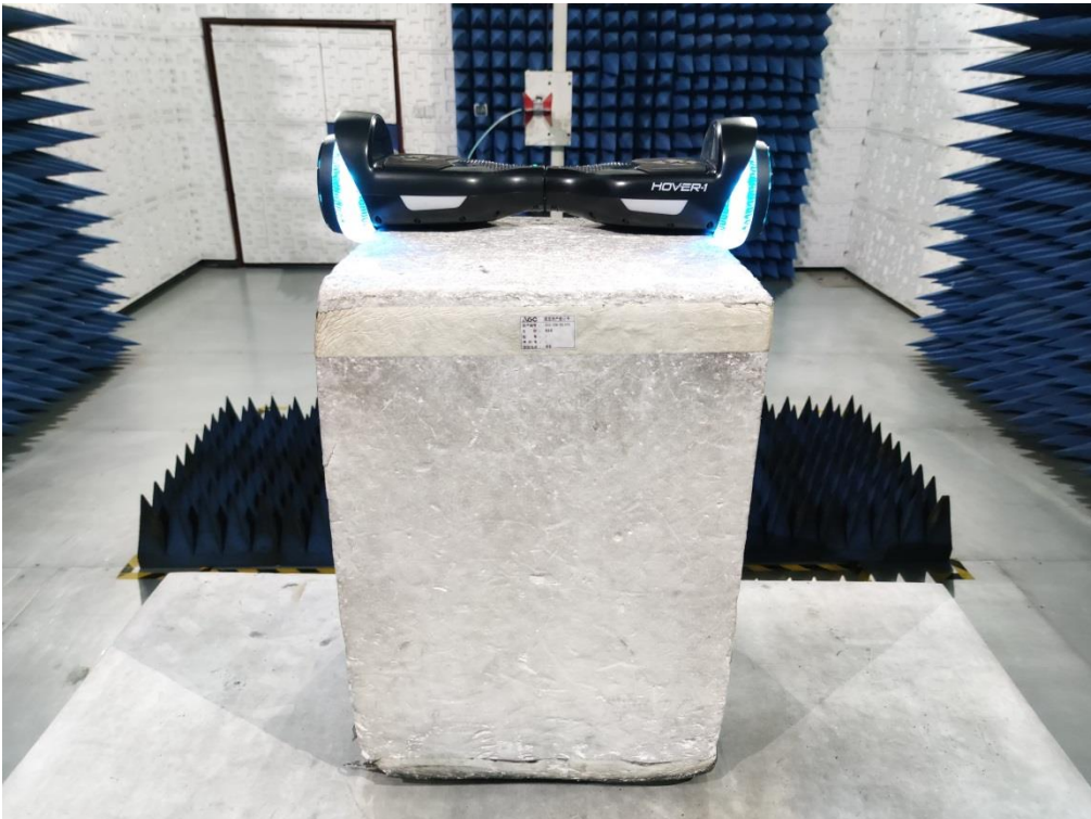
RADIATED EMISSION TEST SETUP ABOVE 1GHz
