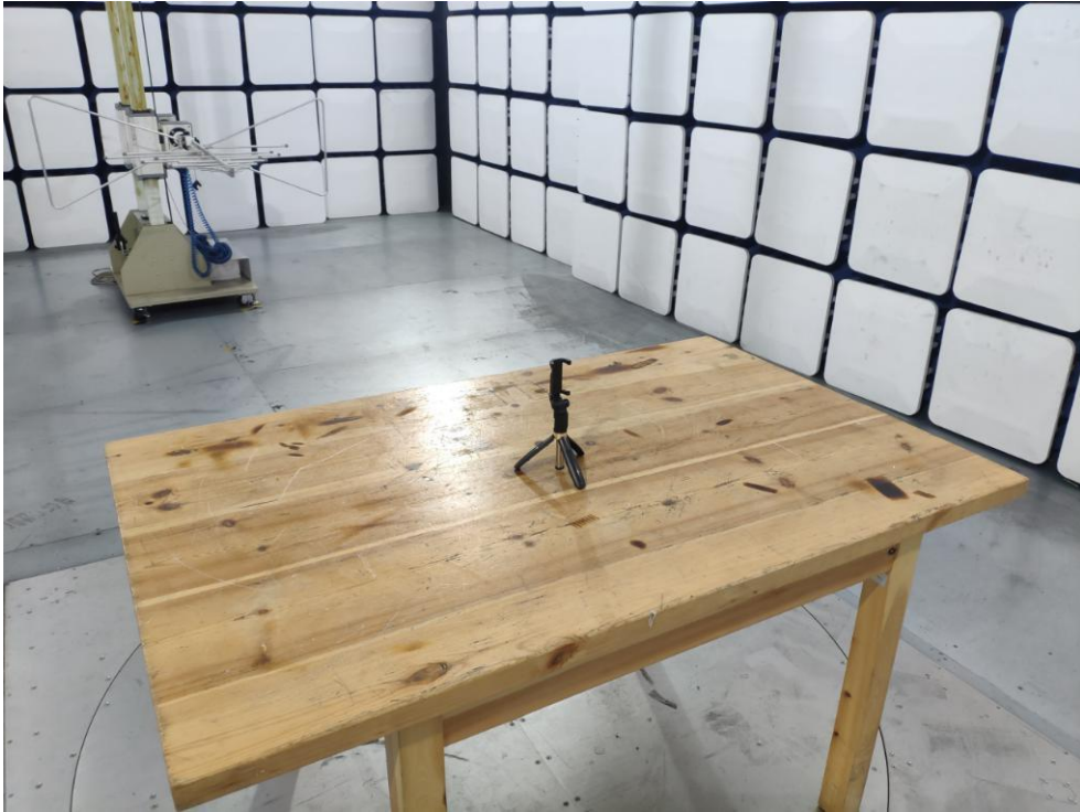
Photo of Radiation Emission Test
