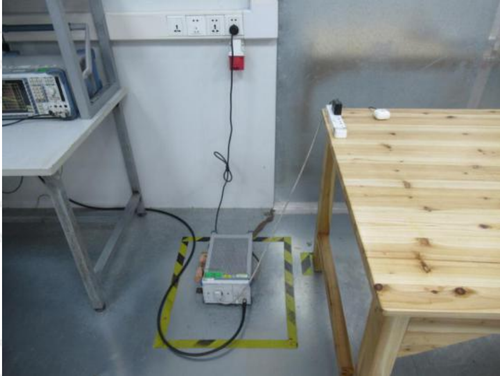
Photo of Power Line Conducted Emission Test
