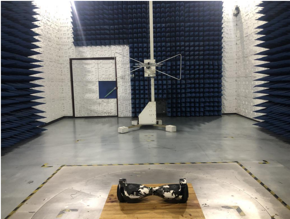
RADIATED EMISSION TEST SETUP ABOVE 1GHz
