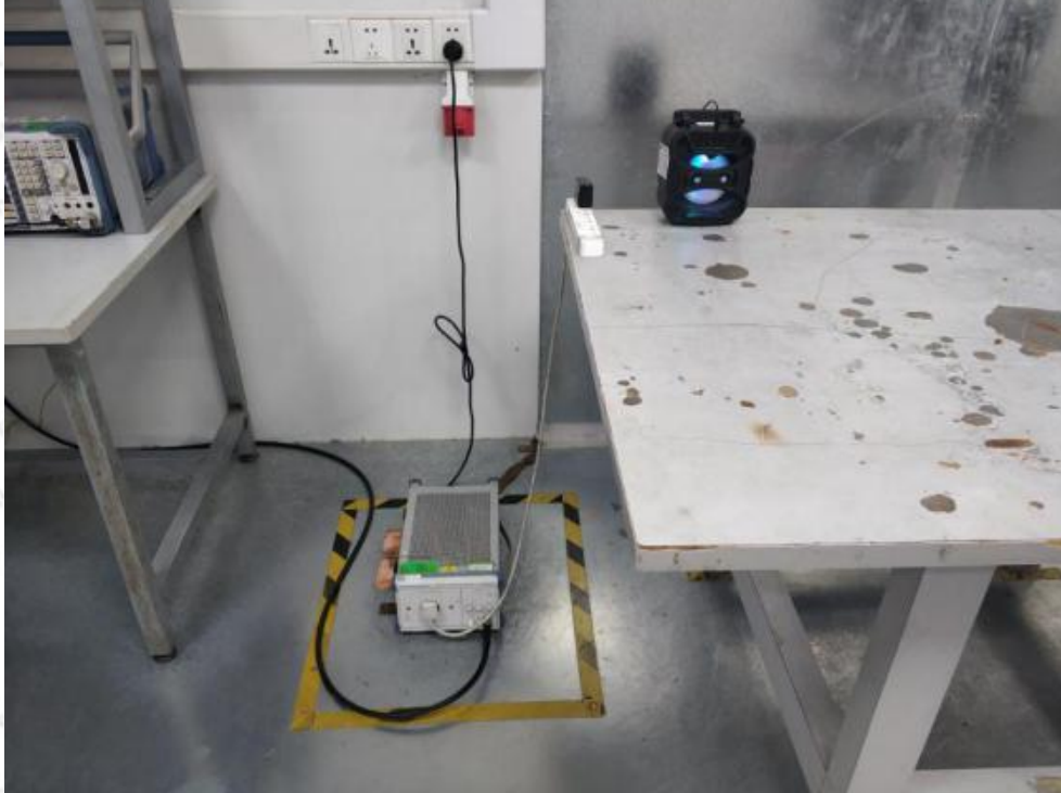
Photo of Power Line Conducted Emission Test
