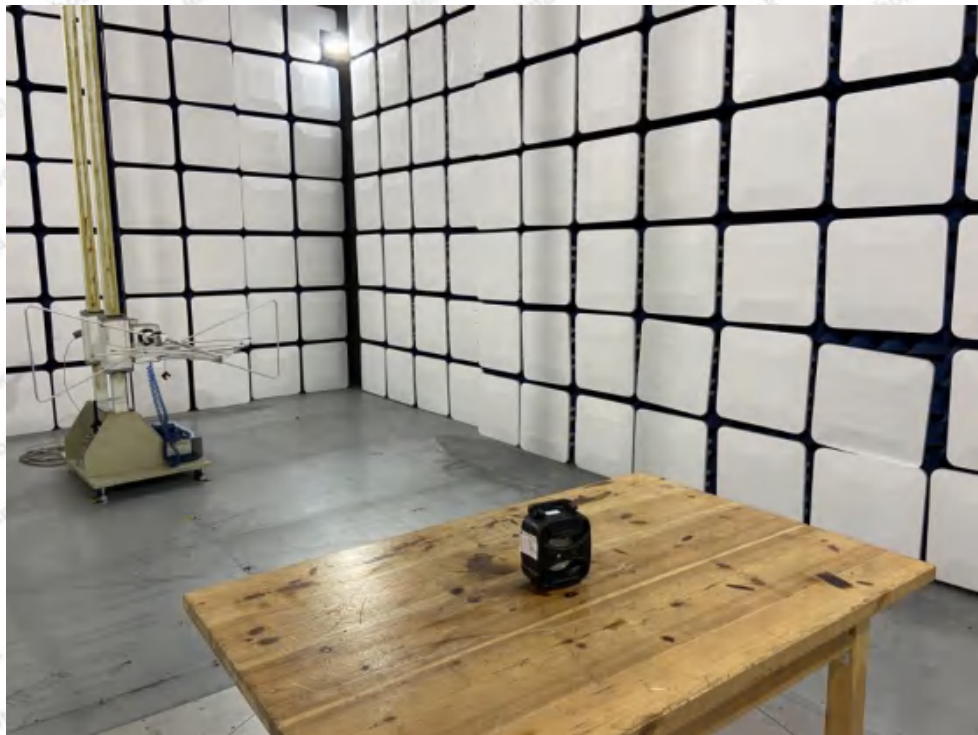
Photo of Radiation Emission Test
