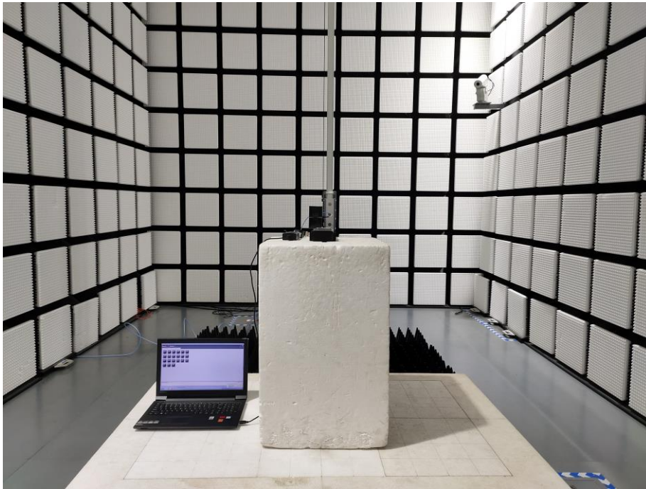
Fig. 3 Radiated emission setup photo(Above 1GHz)
