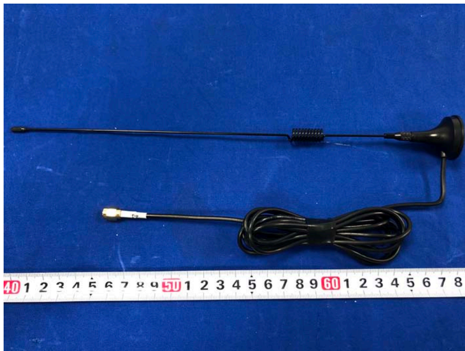
4G Antenna View
