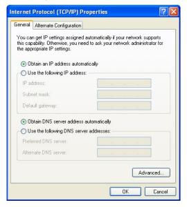
Click "OK", InRouter will allocate an IP address: 192.168.2.x, and a gateway: 192.168.2.1(the default address of IR6x1).
