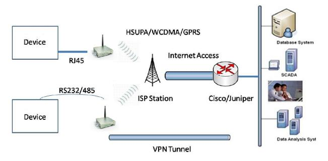
InRouter6x1 series can be used to connect your device (with RS232/485/Ethernet Interface) to internet via GPRS/HSUPA cellular network. Meanwhile, to ensure the security and access, InRouter6x1 series support VPN, enabling remote access and secure data transmission through Internet.
