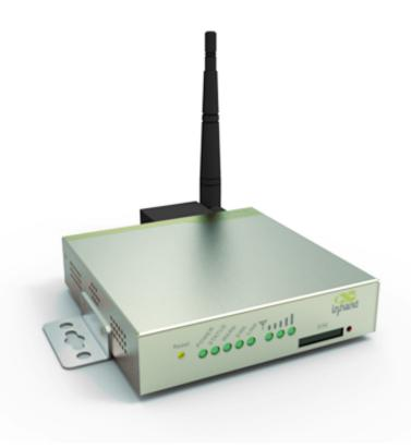
InRouter6x1 series products are Industrial Cellular Router that integrated 2/3G/4G network and virtual private network (VPN) technologies. The products meet fundamental needs of field communication in industry, support international commercial UMTS (HSPA+), LTE networks, and respectively backward compatible with EDGE and GPRS network.
