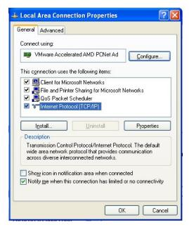
Choose "Internet Protocol (TCP/IP)" and click on "Properties", ensure your PC can obtain IP and DNS address automatically. (Or you can set your PC in the subnet: 192.168.2.0/24, for example, set as IP: 192.168.2.10, Net Mask: 255.255.255.0, Default Gateway: 192.168.2.1)
