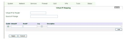
An internal PC's IP can match to a virtual IP, and external network can access the internal PC via this virtual IP address.
