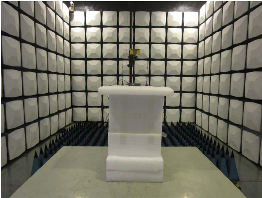
Radiated Emission View (Above 1GHz)
