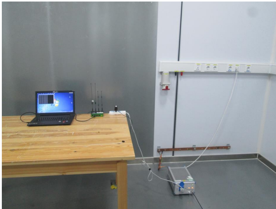
Fig. 4 Power line conducted emission setup photo
