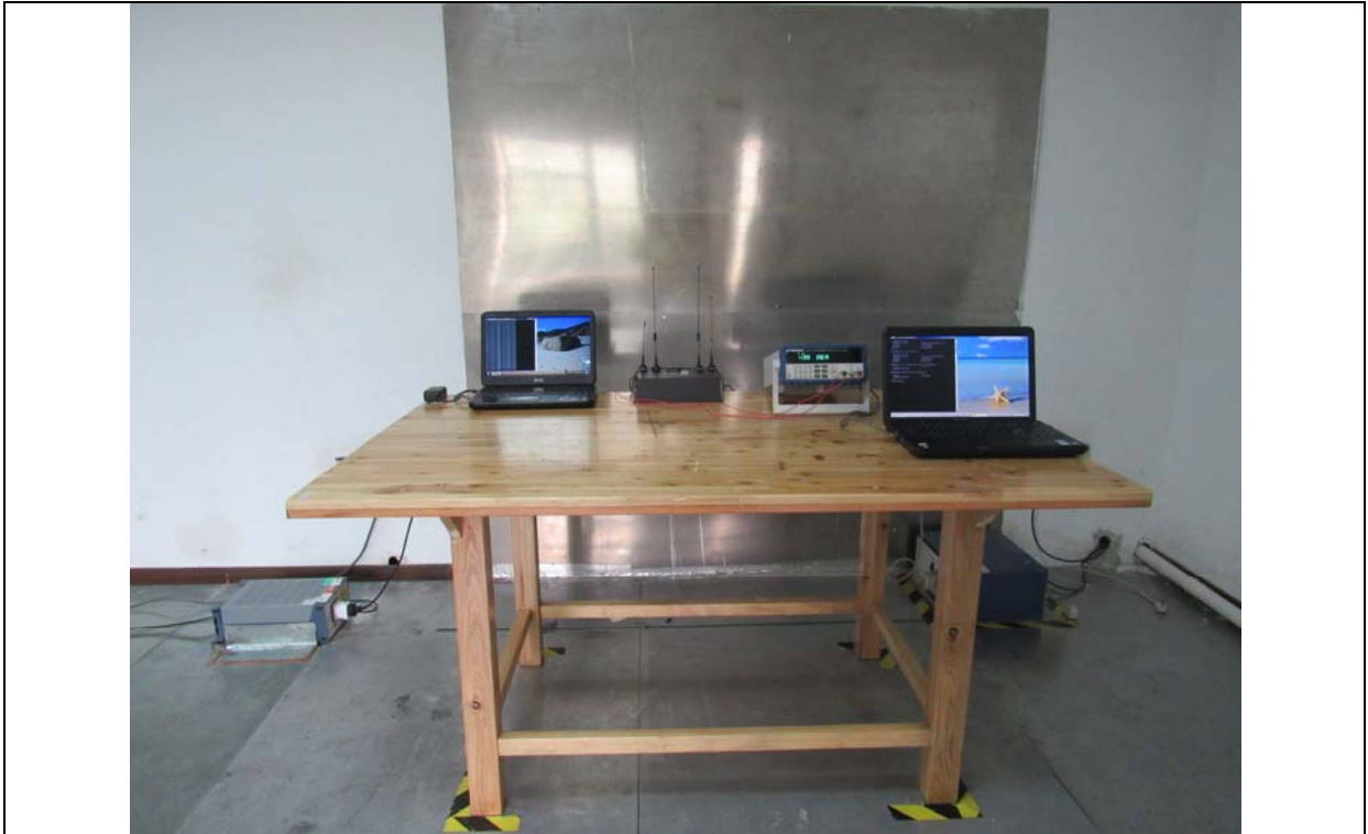
Conducted Emissions Setup Front View
