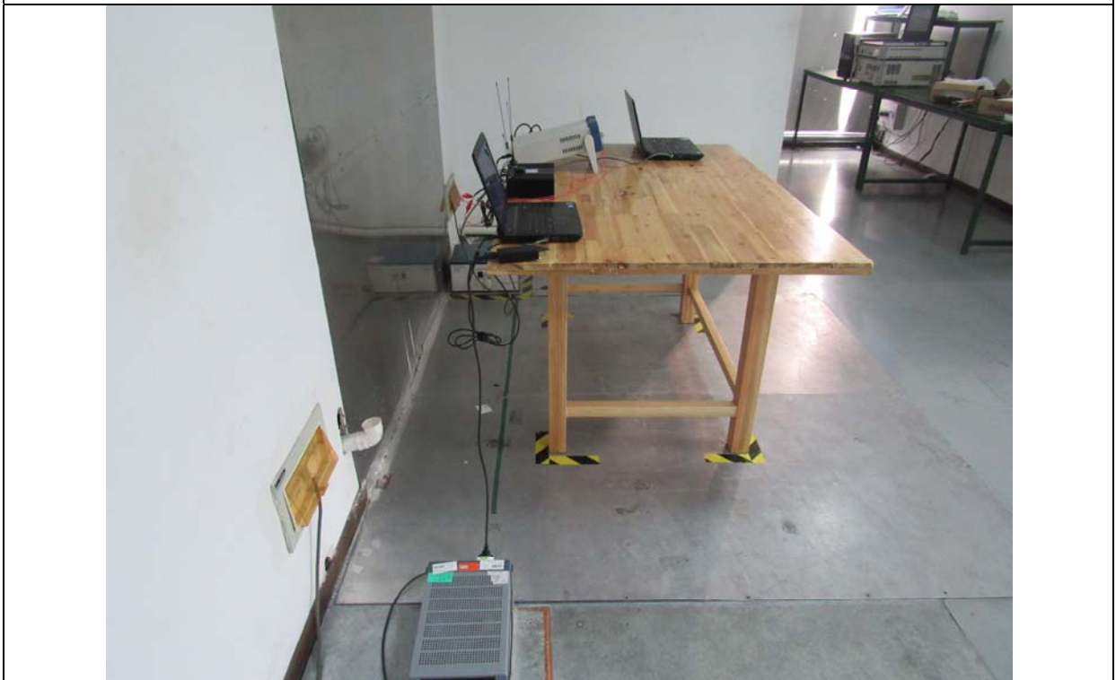
Conducted Emissions Setup Side View
