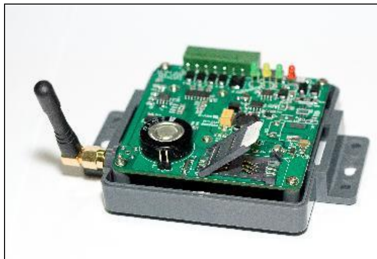
Figure 2-2 Installing SIM card into InDTU332N
