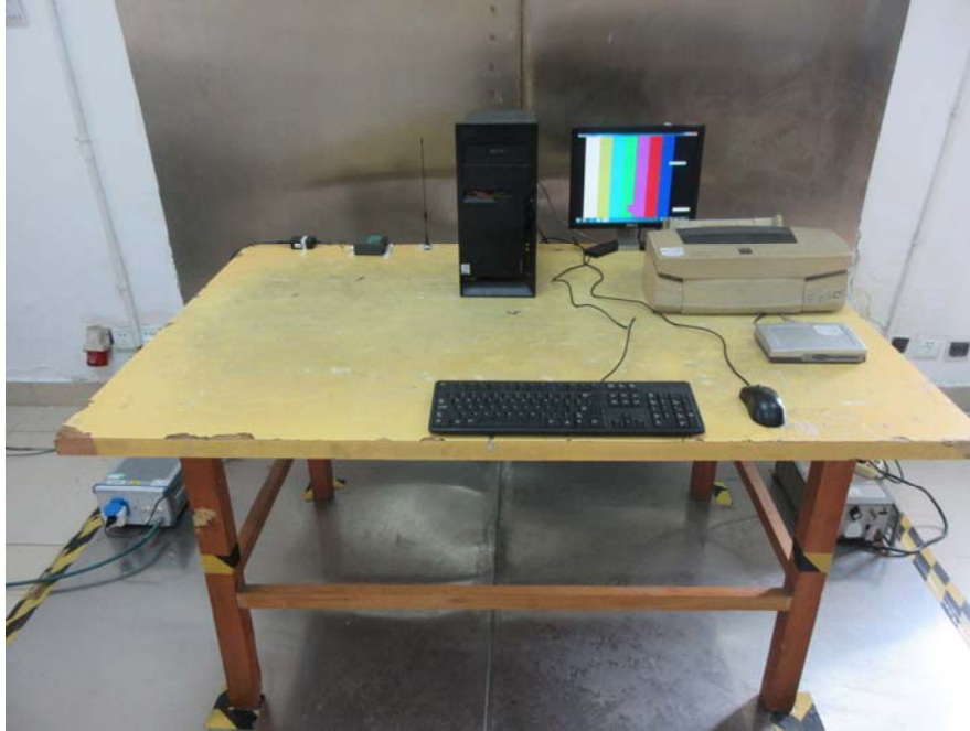
Conducted Emission Test Setup Front View
