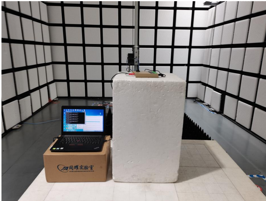
Fig. 3 Radiated emission setup photo(Above 1GHz)
